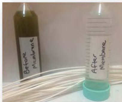
Figure 1. Algae culture before and after filtration with MF membrane.
