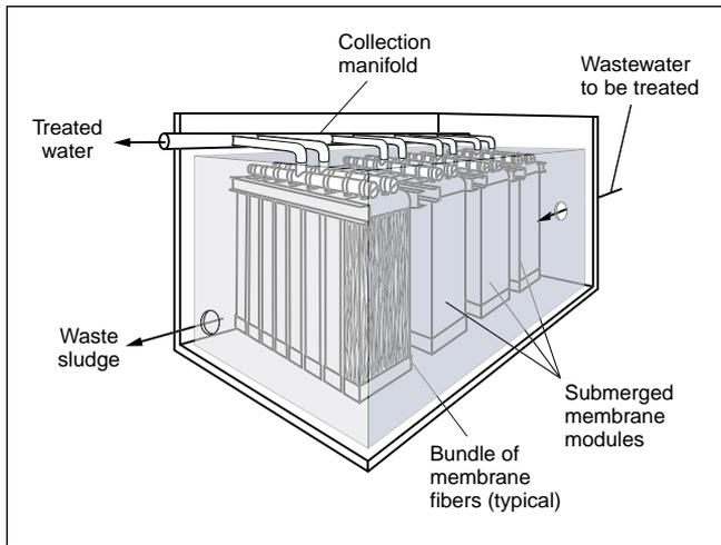
Figure 7. Schematic of a membrane bioreactor for the treatment of wastewater.
