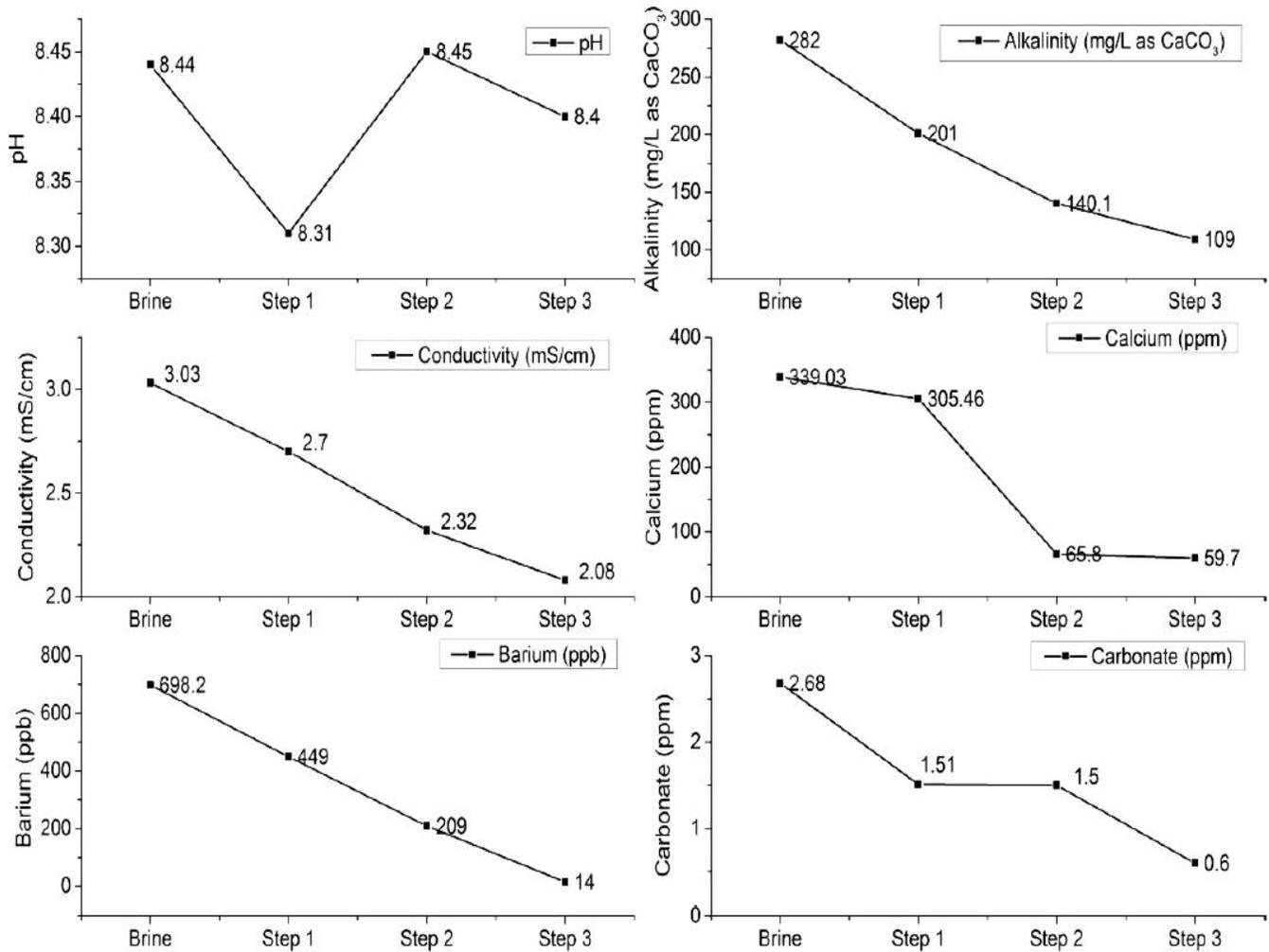
Figure 1 Changes to the composition of the brine after the 3-step treatment process [10]
