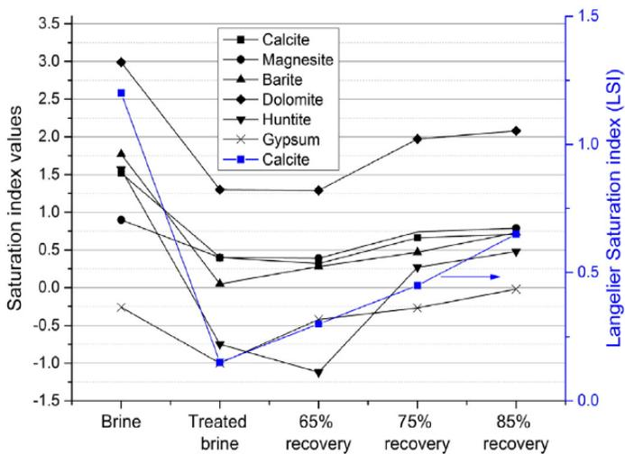
Figure 2 SI values for different recovery rates in the secondary membrane. Also shown are LSI values for CaCO<sub>3</sub> at each stage. The LSI is defined as solution pH value minus the saturation pH value.
