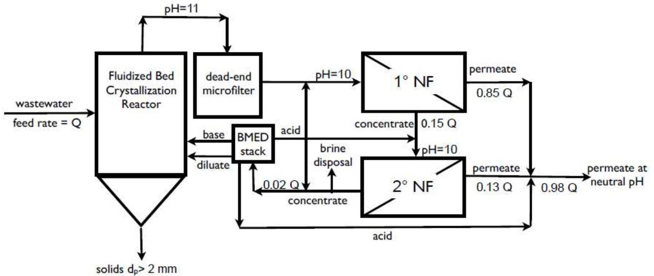
Figure 3 Schematic diagram of proposed treatment process. Approximate volumetric flow rates for different streams are denoted by the fraction of the influent feed rate,  $Q$ . Also shown are approximate pH values for different streams.
