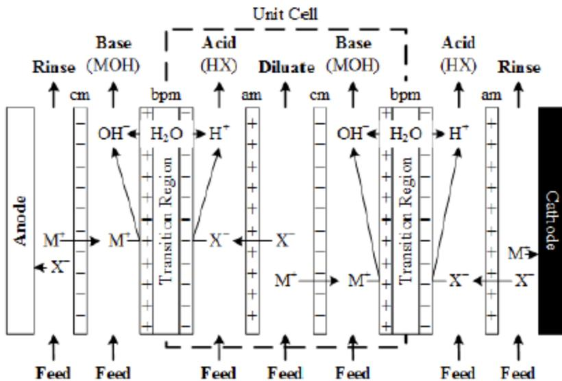
Figure 1 Schematic drawing illustrating the production of acids and bases from the corresponding salts by electro dialysis with bipolar membranes. (Davis, J. R.; Chen, Y.; Baygents, J. C.; Farrell, J. Production of acids and bases for ion exchange regeneration from dilute salt solutions using bipolar membrane electrodialysis. ACS Sustainable Chem. Eng. 2015, 3 (9), 2337–2342.)
