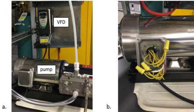
**Figure 2.** (a) The VFD and pump, and (b) a picture of the hardwired electrical connections to the pump.
