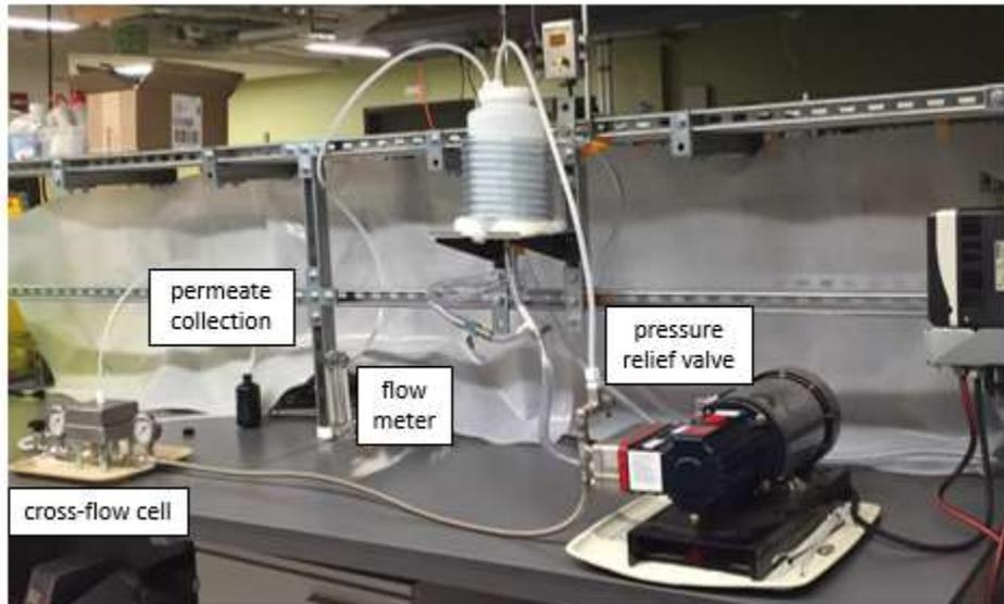
**Figure 4.** The cross-flow system in its entirety.
