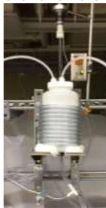
**Figure 3.** The feed tank, with inlet and outlet connections, a chilling coil, and a stir rod.
