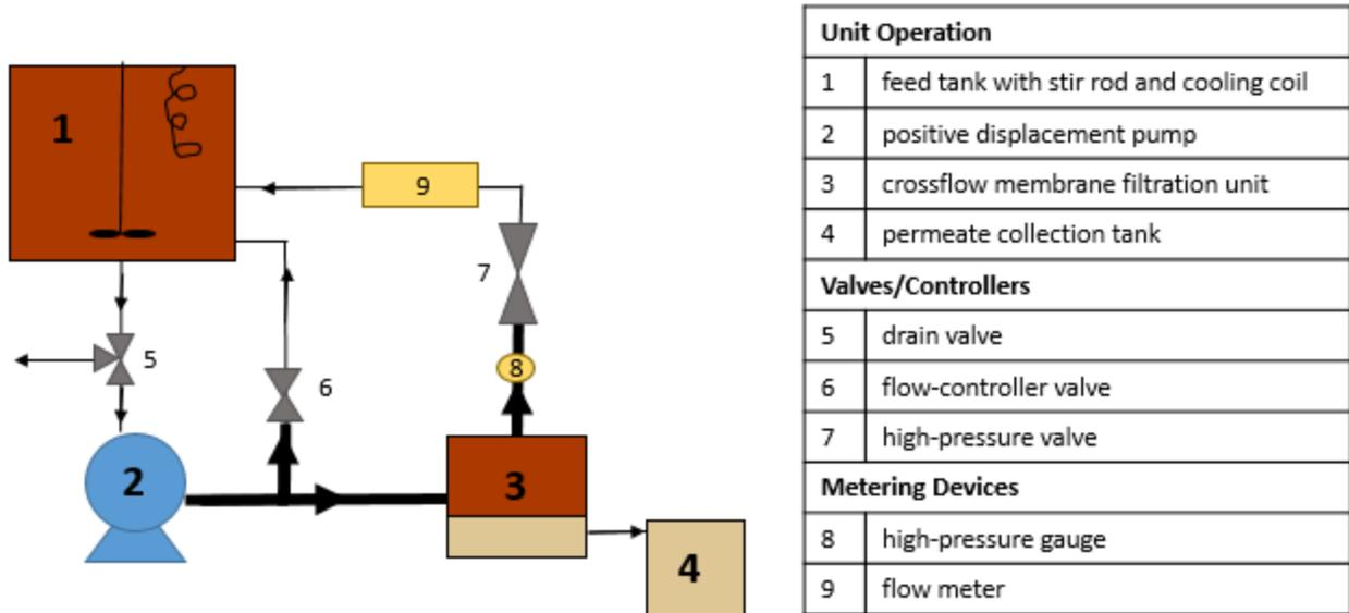
**Figure 1.** The schematic of the crossflow filtration system. Thick lines identify high pressure streams. Adapted from Sterlitech.com
