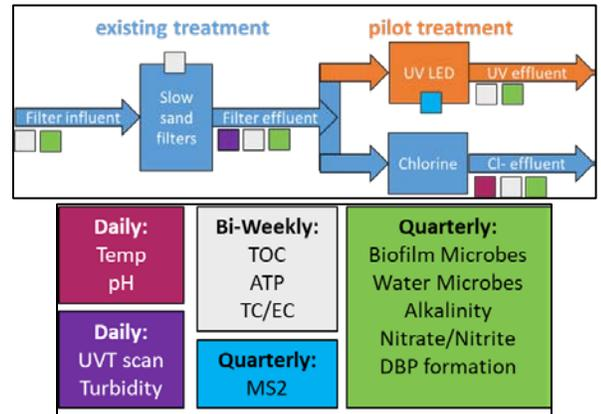
Figure 2 Schematic of existing treatment and pilot UV LED disinfection, showing color-coded sampling locations and schedule for the pilot study.
