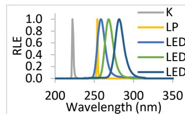
Figure 1 - Relative Lamp Emission (RLE) spectra for the KrCl excimer lamp (K), low pressure mercury lamp (LP), and light emitting diodes (LEDs) used in this study.
