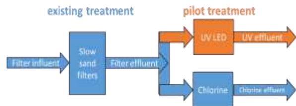
Figure 2 - Local small system drinking water treatment (existing and pilot).
