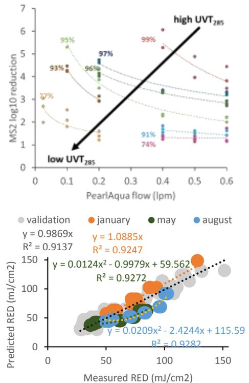
Figure 3 – MS2 disinfection performance of the UVLED reactor at the bench (first panel) and in the field (second panel). Reduction equivalent dose (RED) is the collimated beam UV Dose that achieved equivalent log<sub>10</sub> reduction of MS2 in the flow through reactor. Predicted RED was modeled using bench data in the first panel by a combined variable approach<sup>15</sup> for comparison to measured field data in the second panel.
