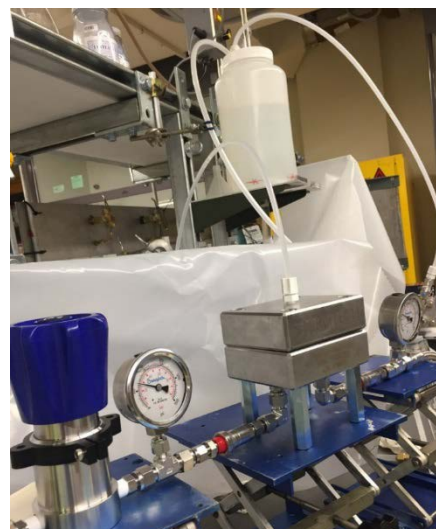
Figure 1. The cross-flow filtration system assembled in our lab.
