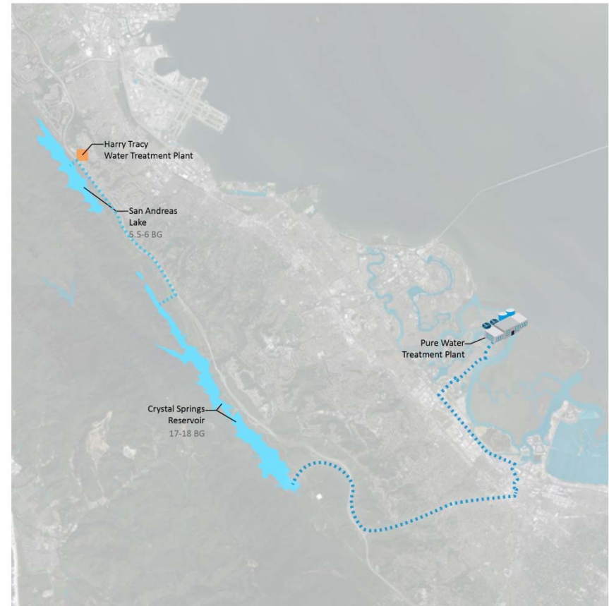
Conceptual Pure Water Treatment Plant - Alignment 2
