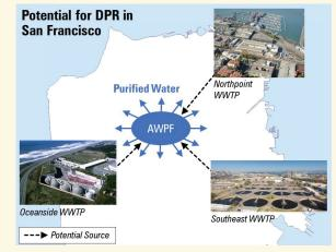
DPR treatment facilities for treated drinking water augmentation could source water from any of San Francisco's three wastewater treatment plants.
