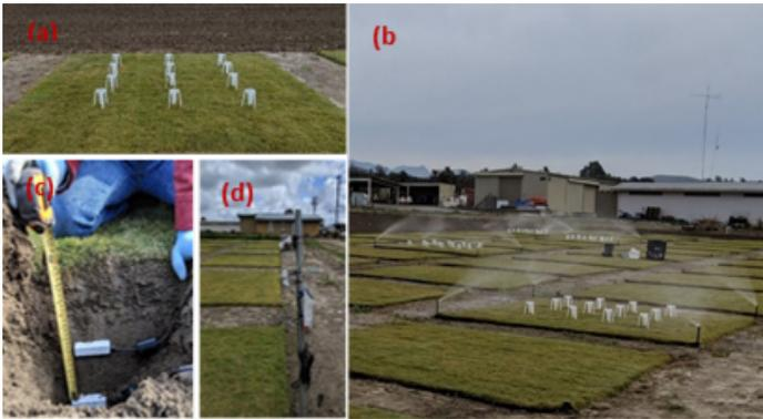
**Figure 2.** Catch cans used for irrigation uniformity test (a), uniformity test at the plots (b), TEROS 12 sensor during installation (c), and setup for continuous canopy spectral and temperature data measurements. (d).
