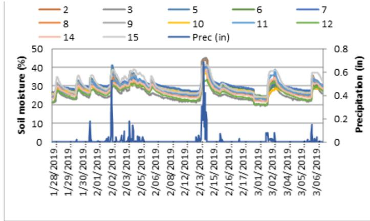
**Figure 4.** Hourly average soil moisture data from Acclima TDT sensors for 12 plots against precipitation data collected from CIMIS #75.
