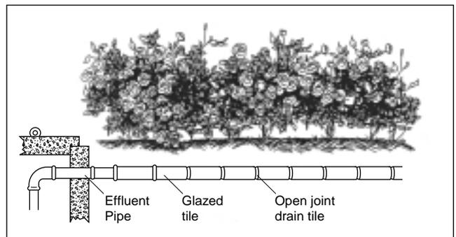
Figure 6. Distribution of effluent from a privy into top soil (after Lumsden et al., 1915).
