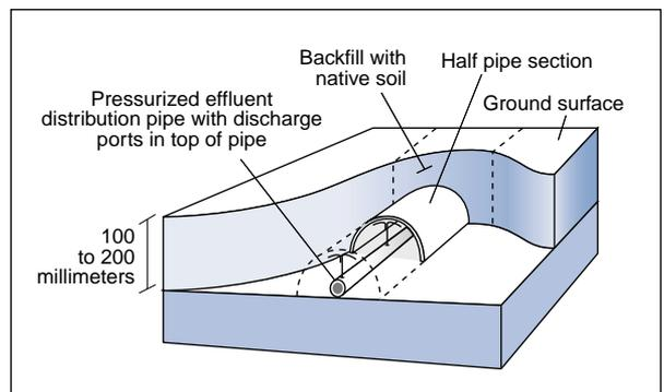
Figure 5. Shallow gravelless pressure dosed adsorption field.
