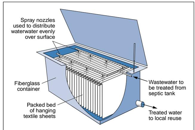
Figure 3. Schematic of textile filter for the treatment of septic tank effluent.
