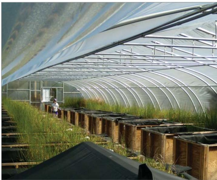
*Figure 3. Mesocosm for studying controlled release of nanomaterials. Photo provided by Dr. Benjamin Espinasse, Duke University.*
