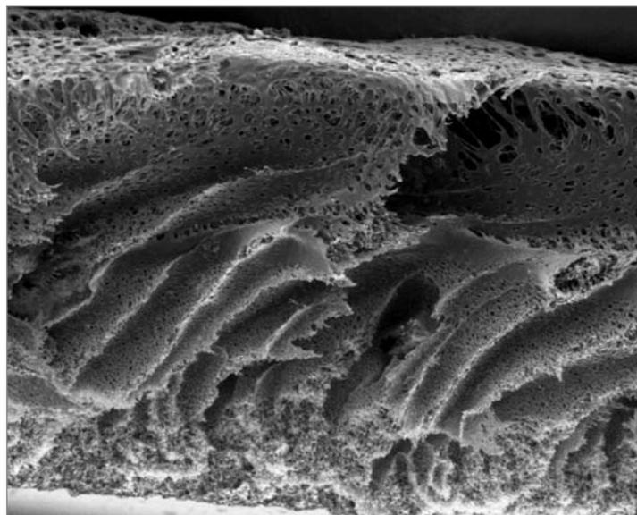
Figure 1. Membrane reinforced with carbon nanotubes. Image provided by Dr. Elif Soyer, Duke University.
