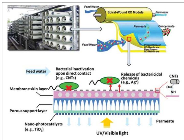
Figure 8. Detail of nanotechnology-enhanced multifunctional membranes for water treatment (Qu et al., 2012).
