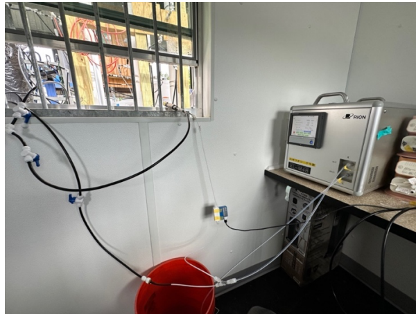
Photograph 2 – Online monitoring system set up at the DPR pilot. RO Permeate is used as the dilution water for 0.2 mL/min of final effluent regulated by a pressure relief valve.
