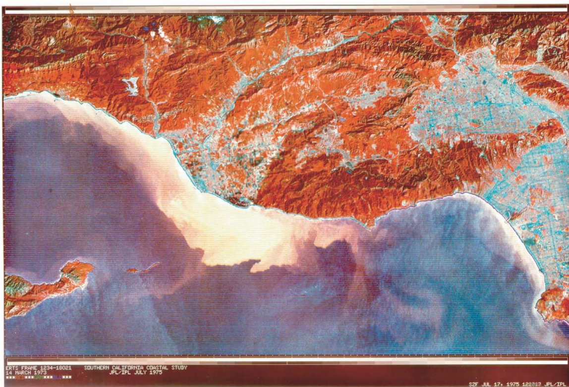
Figure 7: LANDSAT multi-spectral scanner image of suspended particulate across the Southern California Bight due to dispersion of river wash load particulate following a Pacific storm on 14 March 1975.
